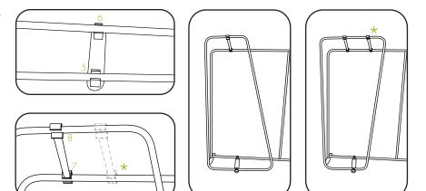
\*If wider end of Wing frame is on top, secure with two Wing bars.
